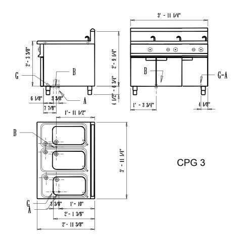
A - water supply connection  $\phi$  1/2" B - water outlet connection  $\phi$  1"
