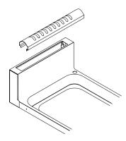
Figure 1b - Removable top flue grid assembly
