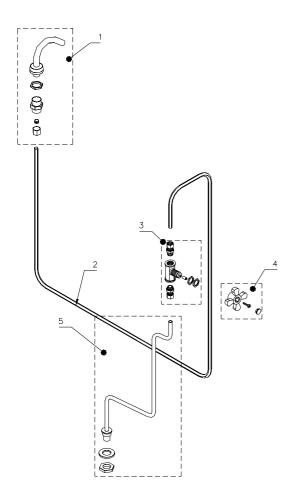
1 Water supply jet 2 Cock to jet pipe 3 Water inlet cock 4 Water inlet knob 6 Water knob disk 7 Copper pipe from supply to cock Figure 2a – Water supply
